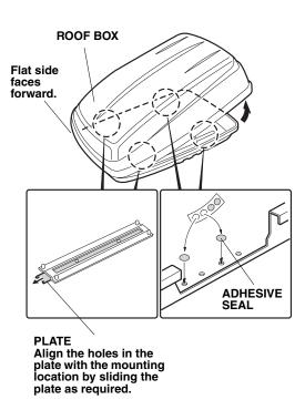
Attach adhesive seals over the four unused mounting holes (two on each side) on the bottom of the box. The seals will help prevent water from entering the roof box. Remove the roof box. 4. Using isopropyl alcohol on a shop towel, clean four brackets B where the small pads will attach. Remove the adhesive backings from the small pads, and attach them to the brackets B.
